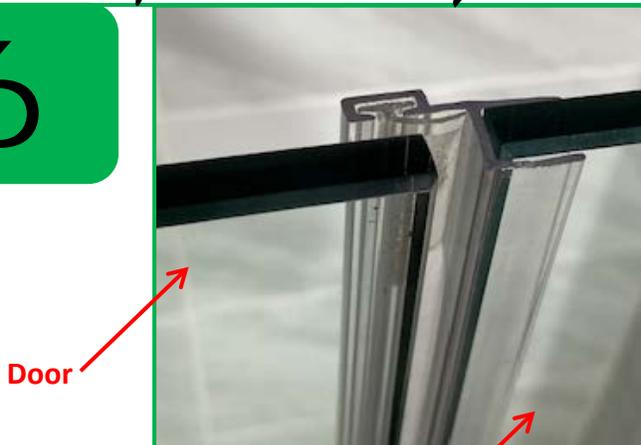
An Optional Acrylic Strike Jamb is available. This clear polycarbonate extrusion presses over the fixed panel and the door closes into the soft wiper blade for increased waterproofing.
